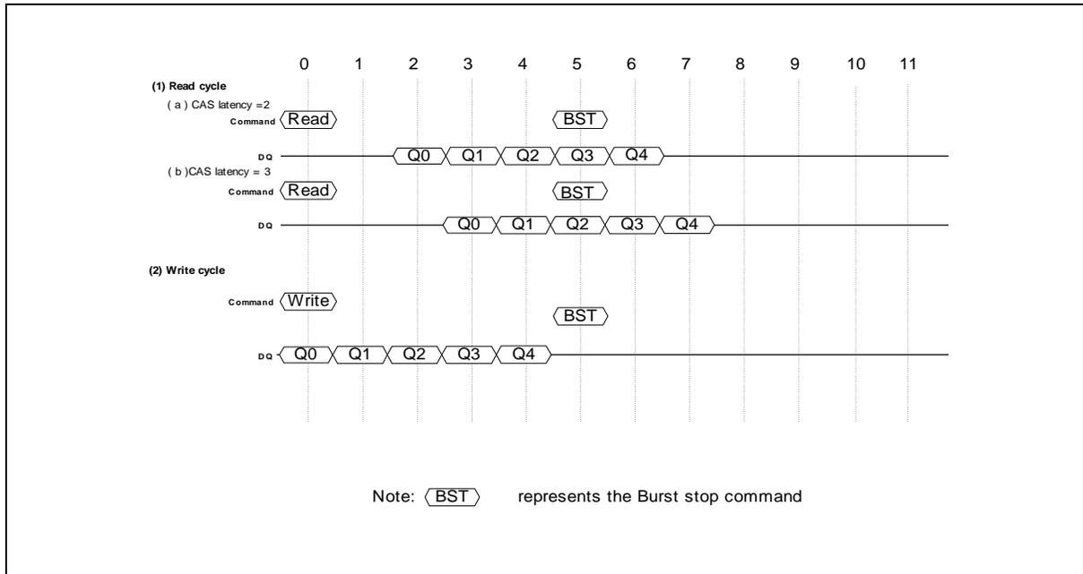
11.20 Timing Chart of Burst Stop Cycle (Precharge Command)
