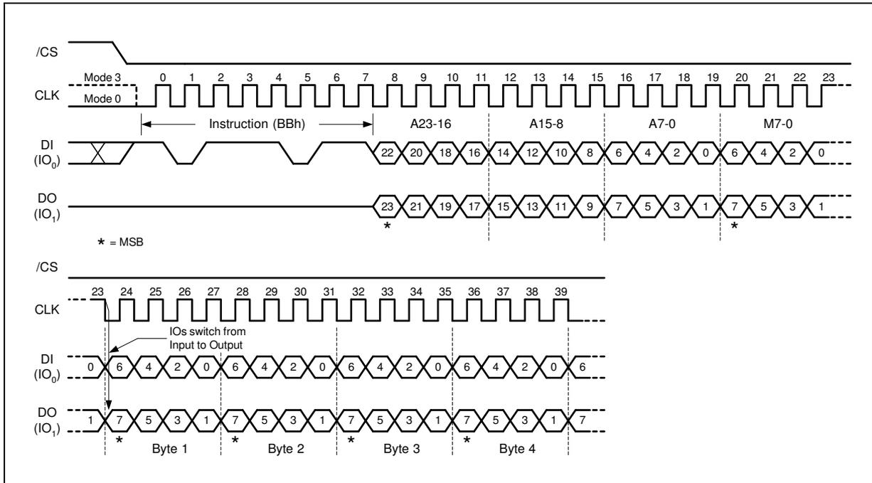
Figure 22. Fast Read Dual I/O Instruction (M5-4=F<sub>x</sub>h)
