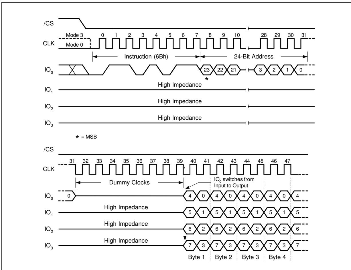
Figure 20. Fast Read Quad Output Instruction
