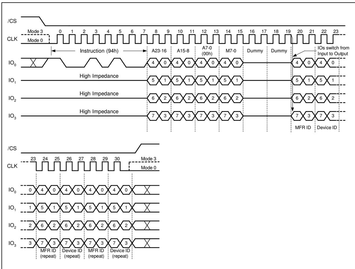
Figure 41. Read Manufacturer / Device ID Quad I/O Instruction
