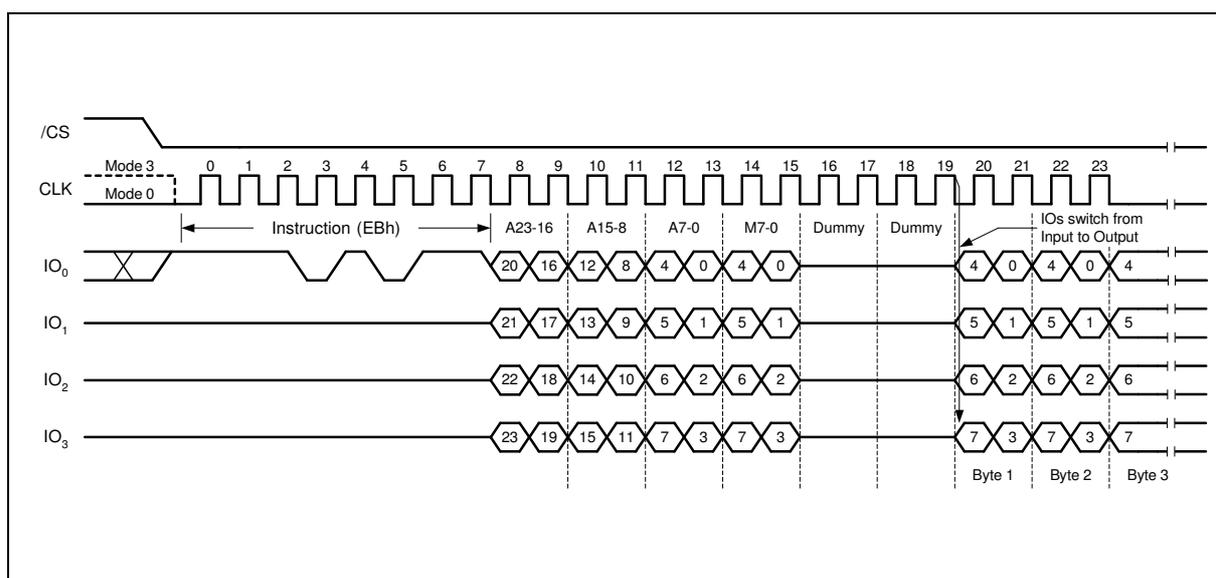
Figure 24a. Fast Read Quad I/O Instruction (M5-4=F<sub>x</sub>h)
