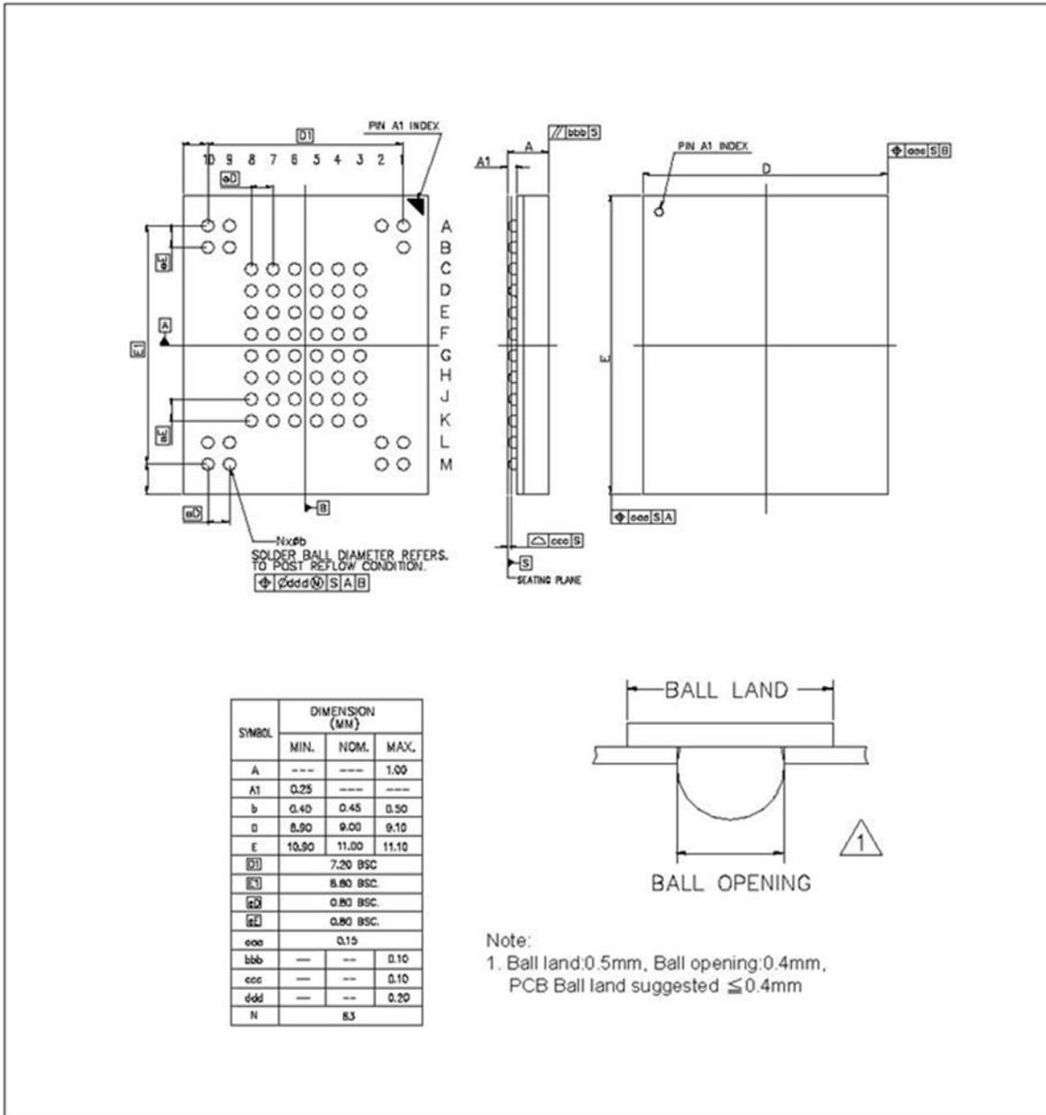
Figure 13-3 Fine-Pitch Ball Grid Array 63-Ball (9x1mm)
