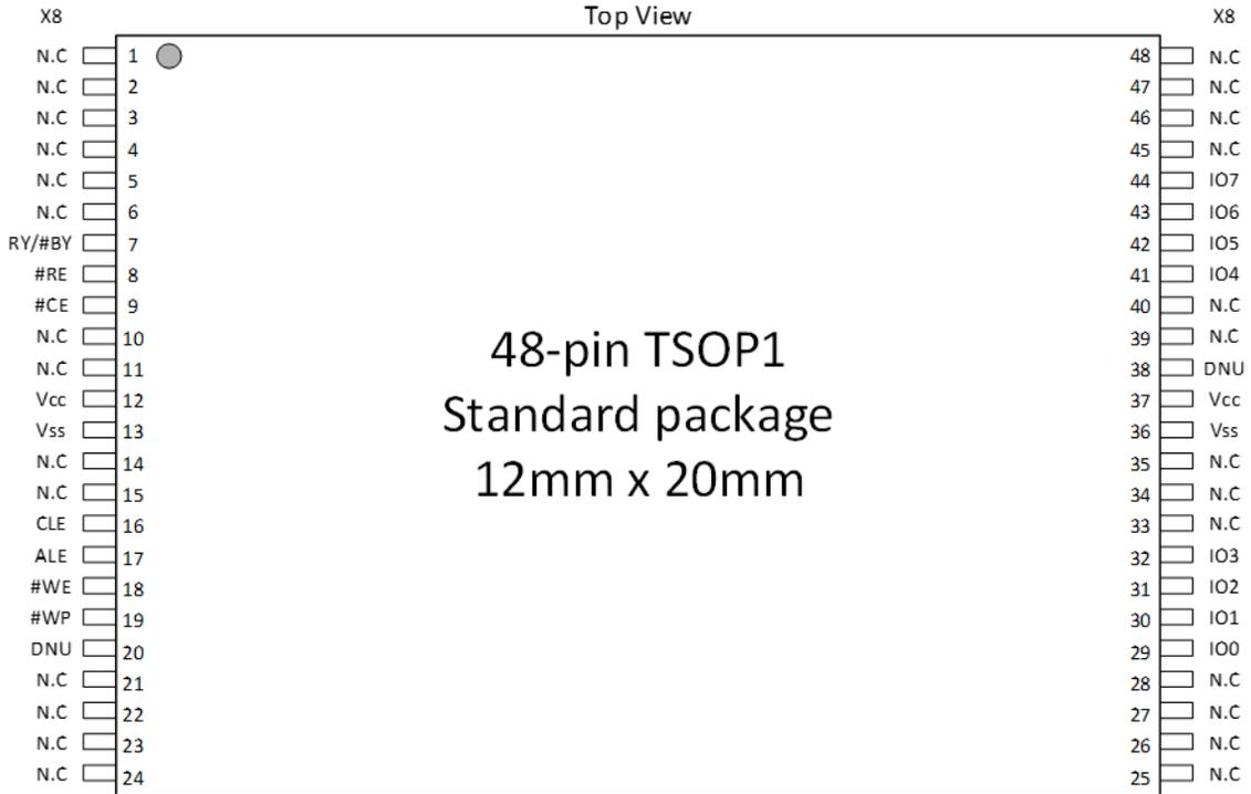
Figure 3-1 Pin Assignment 48-pin TSOP1 (Package code S)
