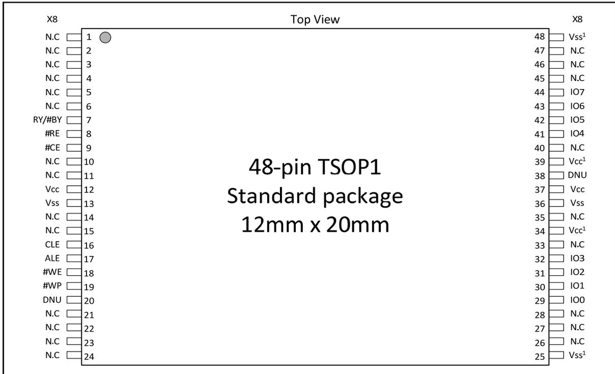
Figure 3-1 Pin Assignment 48-pin TSOP1 (Package code S)
