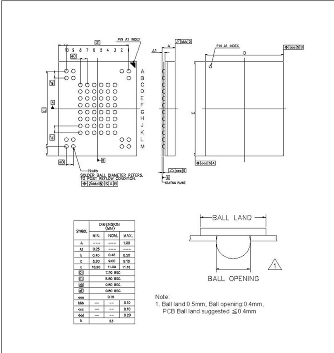
Figure 13-2 Fine-Pitch Ball Grid Array 63-Ball
