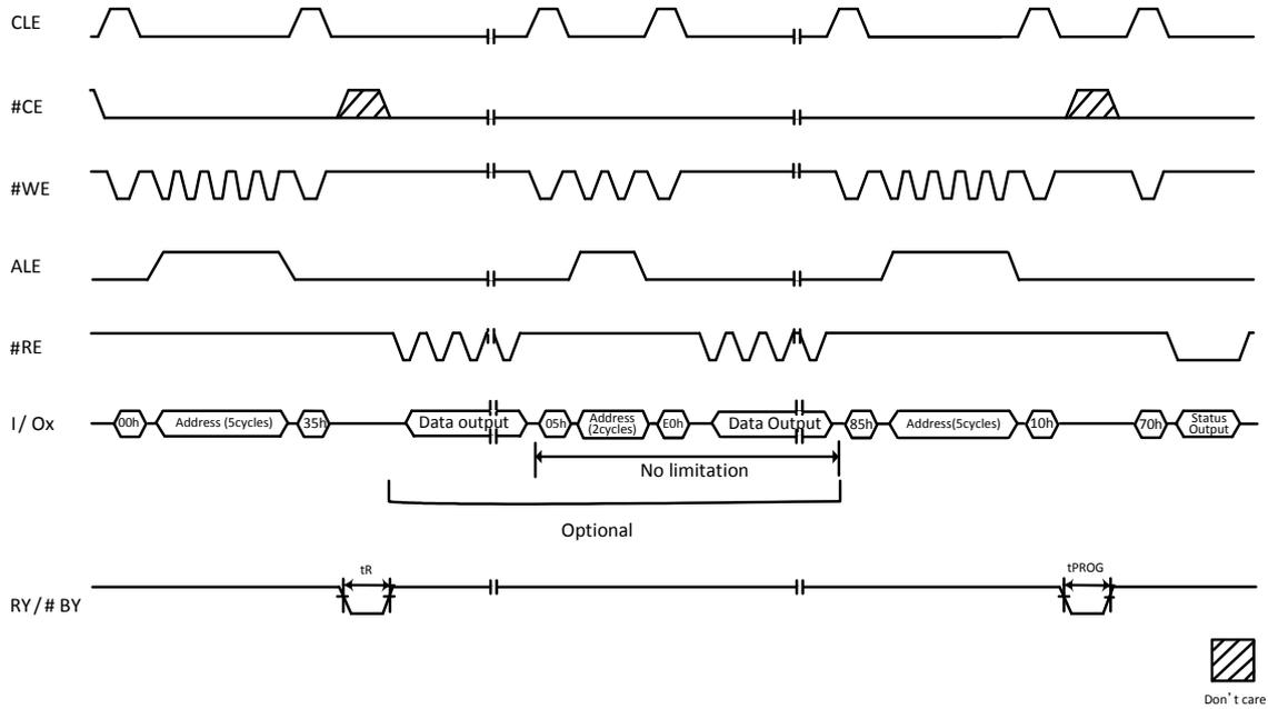
Figure 9-18 Program for copy back Operation
