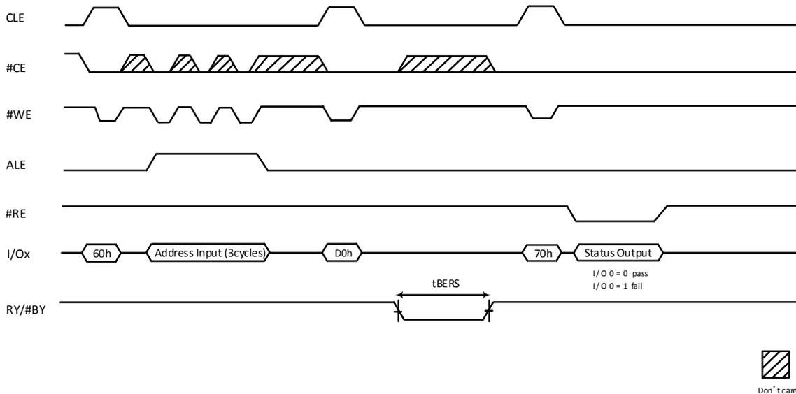
Figure 9-23 Block Erase Operation
