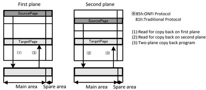
Figure 9-22 Two Plane Program for copy back
