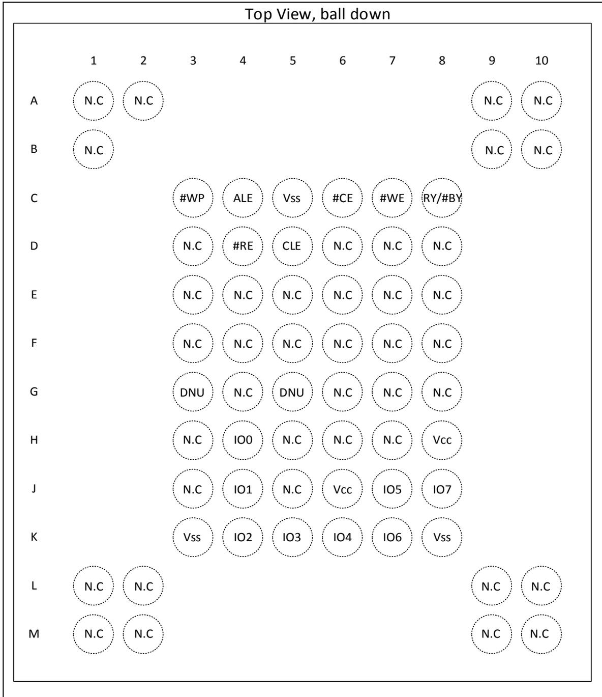
Figure 3-2 Pin Assignment 63-ball VFBGA (Package code B)
