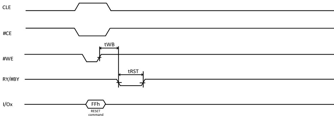
Figure 9-25 Reset Operation
