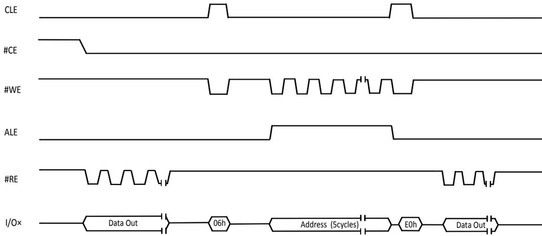
Figure 9-7 Two Plane Random Data Read (06h-E0h) Operation
